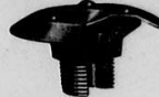
The International Tobin Bronze Umbrella Distributing Nozzle. The amount of wash water distributed by each nozzle is governed by the diameter of the orifice in the body. The cone-umbrella cap assures perfect distribution.
