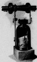
International Pressure Coagulant Feeder with Venturi Proportioner
